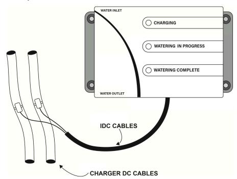
Figure 11. IDC Cables connect the WaterGenius to the Charger DC Cables
