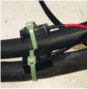
Figure 12a. Push the IDC into the copper core of the Charger DC Cable
