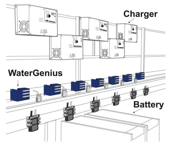
Figure 5. Water Genius mounted to Battery Charger Racking
