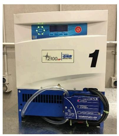
Figure 4. WaterGenius mounted to front face of Battery Charger
