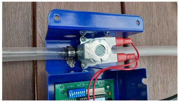
Figure 10. Secure hoses to Solenoid Valve with included Stainless Steel Clamps
